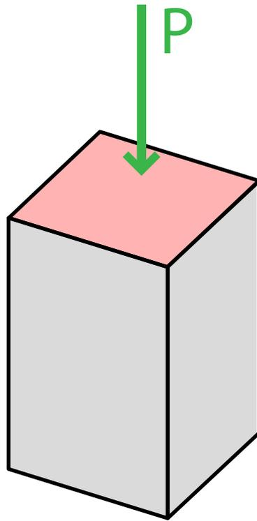
The sample strains and deforms into a compressed state, shortening along the axis of the force.
