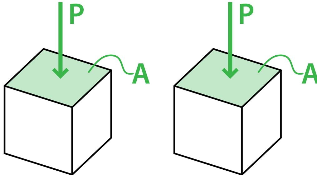
If one of those material samples has a cross-sectional area of 4 in<sup>2</sup>, and a force of 1000 lbs compresses it, the material has a stress of:
