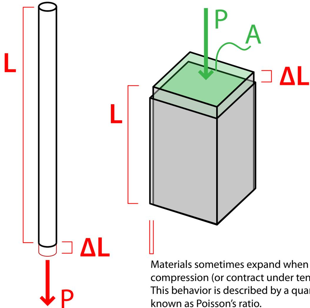
Materials sometimes expand when under compression (or contract under tension). This behavior is described by a quantity known as Poisson's ratio.
