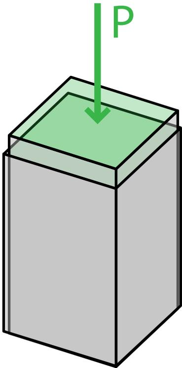
Force is applied to the cross section of a material sample. This forms a compressive stress in the material.
