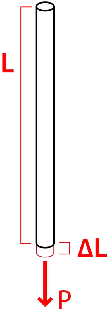
Given  $f_{\text{allow}} = 22$  ksi and  $P = 5,000$  lbs, calculate the minimum cross sectional area for a steel cable.
