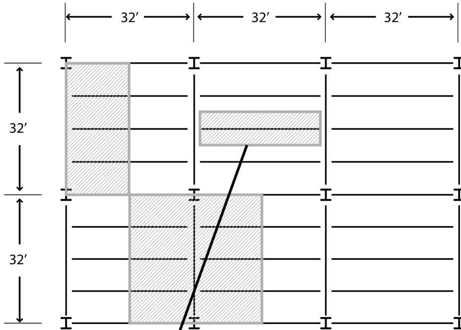
Tributary areas for various beams and girders in a generic steel grid.
