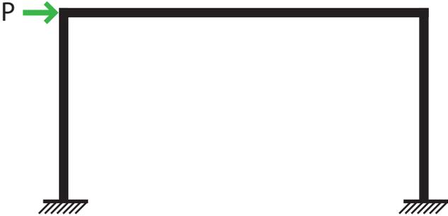
The deformation of the frame itself results in a number of points of inflection, typically one in each member. The locations of these points is a determiner of the relative stiffness of columns and beams.
