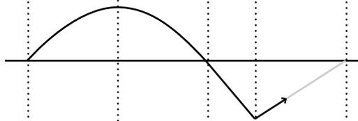
The shear doesn't change along the range from B to the end, so the moment diagram has a constant, negative slope. Graphically, it is a straight line that points downward.
