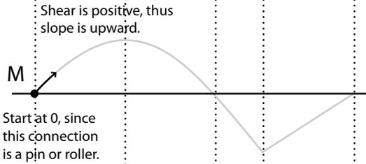
The shear decreases, which means the slope gets increasingly flat, until the shear reaches zero, where the moment flattens out and points horizontally.
