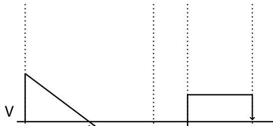
Given the shear diagram, **draw the moment diagram**. The value of the shear diagram is the slope (rise/run) of the moment diagram.
