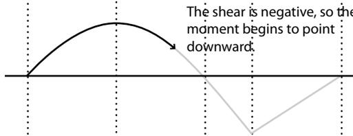
The shear doesn't change along this range, so the moment diagram has a constant, negative slope. Graphically, it is a straight line that points downward.
